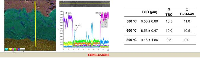
The TBC remained intact and adherent to the Ti-6AI-4V alloy under all test conditions. The microstructural analysis revealed that the Ti-6AI-4V experienced grain growth with increasing temperature; however, this effect was less pronounced with the TBC, demonstrating its effectiveness in protecting the substrate against cyclic oxidation. These results confirm the reliability of the TBC system in enhancing the high-temperature performance of Ti-6AI-4V alloys.
