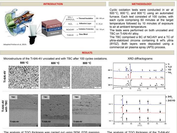
The analysis of TGO thickness was carried out using SEM, EDS mapping, and EDS line scan.
